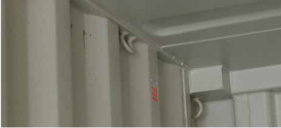
Lashing points (inside a standard container) on the roof, corner post and the small holes for compensation of air pressure.
