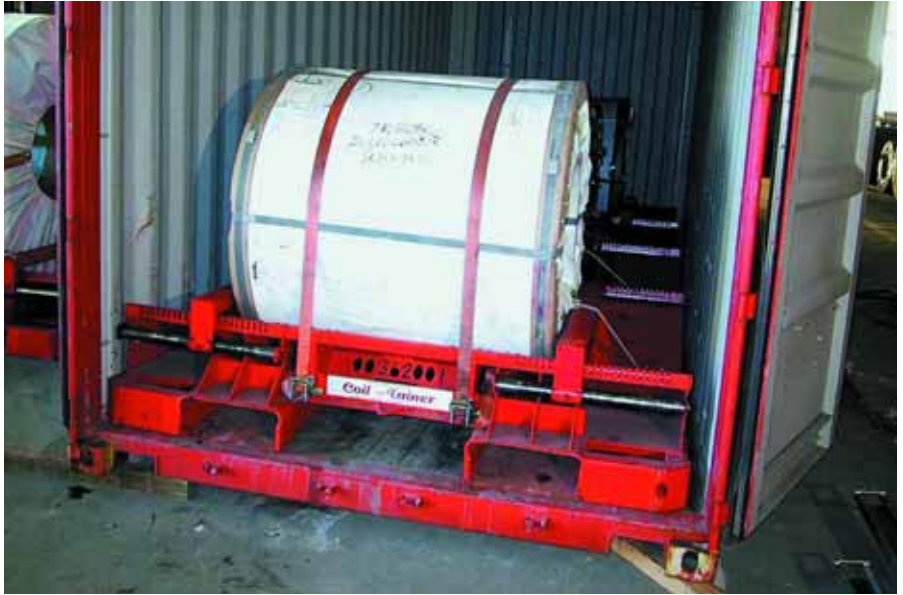
Steel coils secured on a cradle from CoilTainer.
