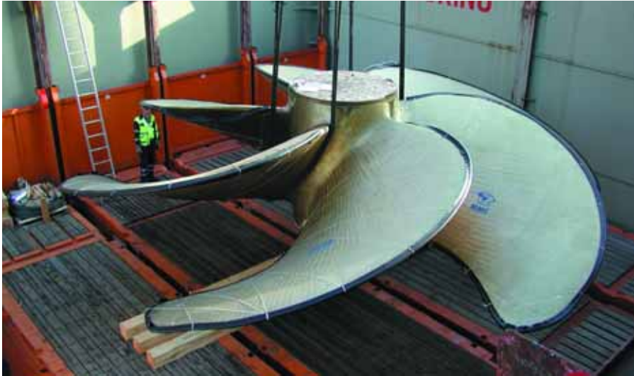
Loading of a large ships propeller of 80t. The propeller has a very small contact area to the base; therefore a strong bedding of timber is used. Additional wooden supports below each propeller blade will be added and steel wire to be used for lashing.
