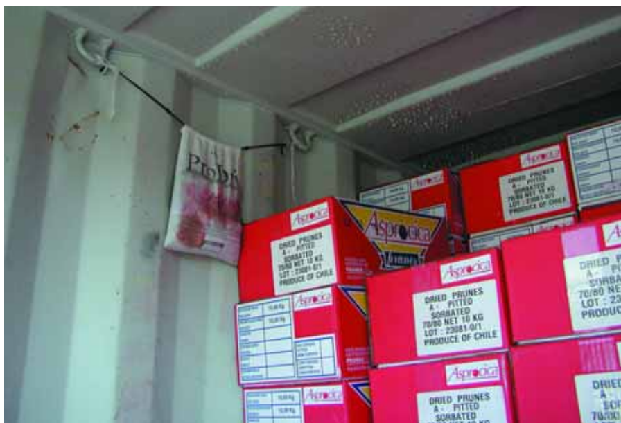
Condensed water at container roof.
