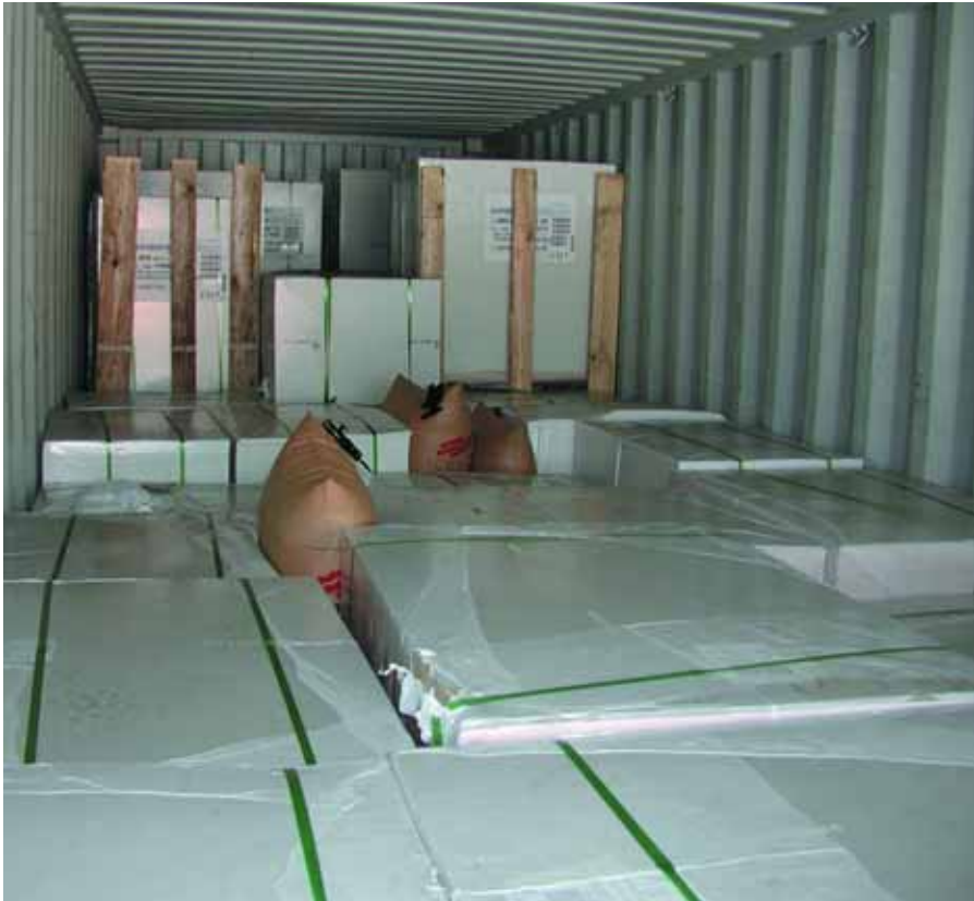
Stowage of non-uniform pallets. The spaces are filled with airbags. The pallets on the second level are blocked against moving forward with 3 pieces wooden dunnage each.
