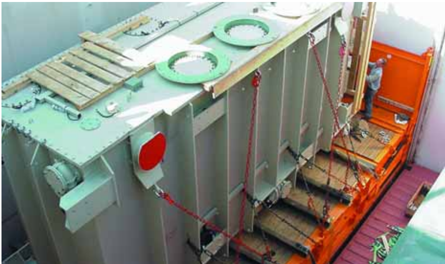
This transformer with an approximate weight of 160t is placed on steel beams and chains are used for lashing.
